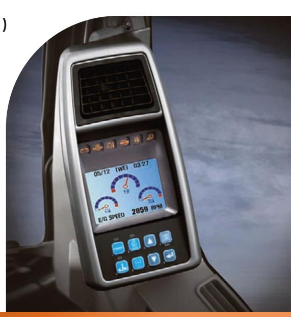
THE YANWA EXCAVATOR HAS AN LCD SCREEN, WHICH ALLOWS THE OPERATOR TO SELECT THE DIFFERENT WORK MODES, EQUIPMENT SPEEDS, AMONG OTHER OPTIONS.
