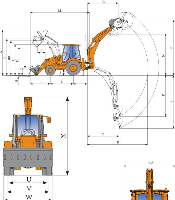
When the machine is used for object handling operations, the backhoe part must be equipped with safety valves (boom, arm and overload warning device) in accordance with EN474-5 and must operate in accordance with the regulations related premises.
